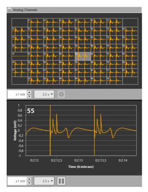
Data display of ECG signals of the atrium, delivered from the 60MEA-SG. You see the overview of all electrode channels above and the single view of channel 55 below.
