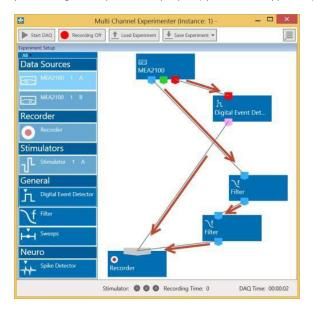
Please consider the rules for connecting the instruments. The Multi Channel Experimenter program allows only connections between output ports at the lower side of the device to the input port on the upper side of the target device. The input and output ports of the devices are color coded for a better assignment of the instruments.
