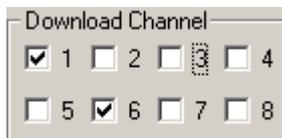
However, the individual download option is influenced by the **Trigger Settings**. To be able to download channels independently from each other, it is mandatory that these channels are assigned to **different triggers**.
