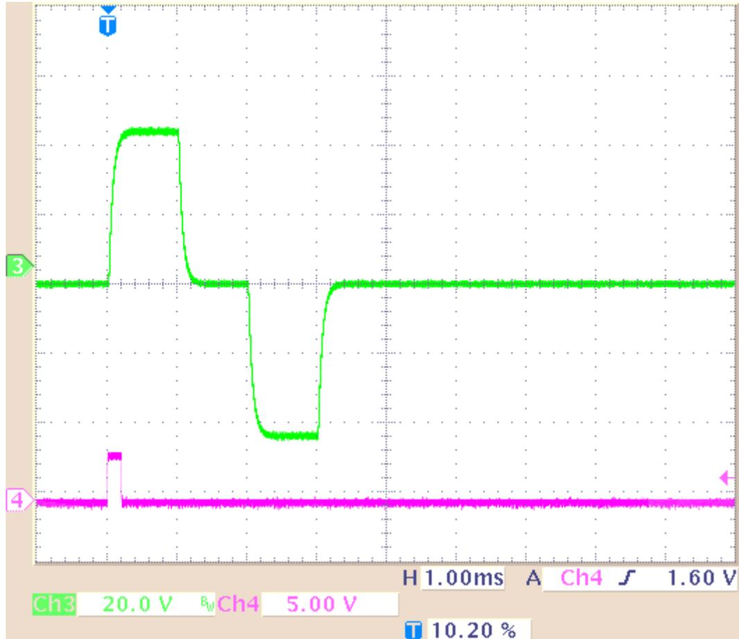
**Result of Example 4:** The current output signal is delivered negligible modified when the duration of the signal and the duration of the interval is long, for example 1 ms.
