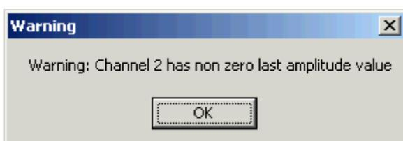
The last voltage / current values of the named channels are not zero. The current / voltage levels are set to **zero** after the last value. The last used values of these channels are **kept** until the STG is stopped.
