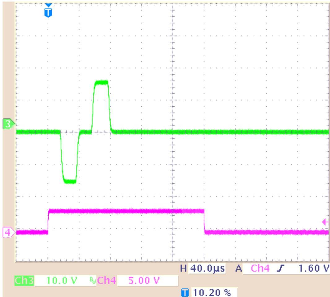
**Result of Example 1:** The current output signal is delivered unmodified without any influence of the length of the pulse with an amplitude of 1600  $\mu\text{A}$  which is at the maximum capacity of the STG 4000 series.
