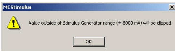
The ASCII file contains current / voltage values outside the STG's range. For example, if the STG's output range is  $+8000$  mV, all values above  $+8000$  mV are set to  $+8000$  mV.
