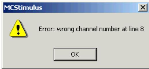
The channel number specification has to precede the data. The channel number either lacks or the specified number does not exist (for example, number 13).
