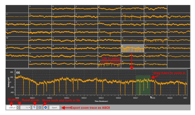
In the Zoom Display, it is possible to zoom in further by dragging a frame around the region of interest. A click on the arrow button will reset the zoom. The data from the Zoom Display can be exported as ASCII (\*.txt file).
