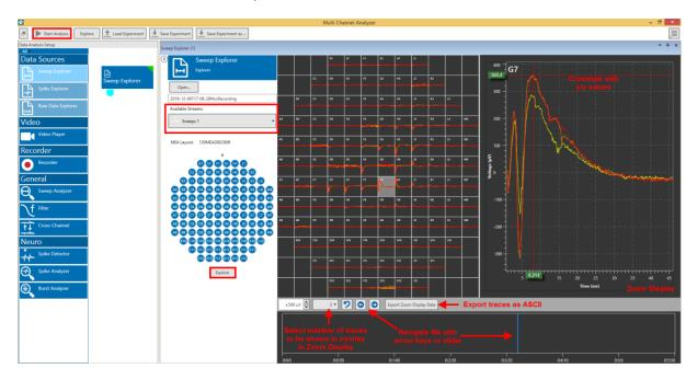
All available data channels of the selected stream in the loaded file will be shown in the layout which was selected during recording. Individual channels can be **toggled** by clicking on them. Deactivated channels will no longer be shown, and not be transmitted to the connected analysis instruments. This can speed up the analysis process.
