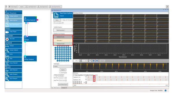
If more than one Trigger data stream is present, select one from the drop down menu Make sure the position in the file is around a trigger before using Explore, or the Sweep window will be empty. If the selected Trigger stream contains more than one type of event, you can define the exact event to be used as trigger source in the Sweeps tool.
