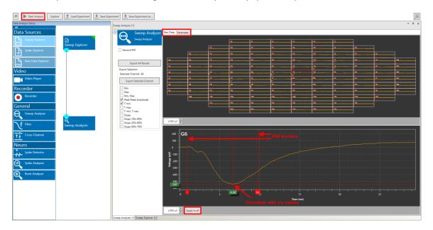
A cross hair is available, which can show x and y values of any specific point in the plot. Once the ROIs are set for all relevant channels, the **Start Analysis** function can start the processing of all sweeps in a file.
