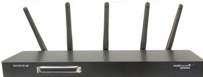
For recording analog signals additionally, please use the receiver W2100-RE-AO with analog output. The 68-pin MCS standard connector provides access to analog data for streaming into third party data acquisition, for example the USB-ME64-System. In double systems it is possible to use optionally one receiver with and one without analog output or both receivers with analog out.
