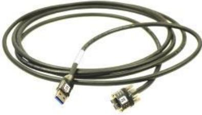
Hint: Make sure that no mechanical forces act on the cable plugs. Do not break off the cable directly after the plugs. This may damage the plugs. Optional: If it is necessary to fix the cable, please use a strain relief with a minimum distance of 50 mm on each plug when installing the cable.
