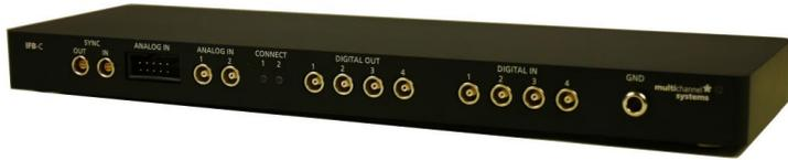
The multiboot interface board IFB-C facilitates operation of all MCS *in vitro* and *in vivo* headstages within the entire 2100 amplifier solution suite. This suite includes: MEA2100-HS, Multiwell-MEA-HS, CMOS-MEA-HS, MEA2100-Beta-Screen-HS, W2100-HS and ME2100-HS. The modular 2100 amplifier solution suite design makes it easy to modify your lab equipment generally with modest hardware upgrade investments.
