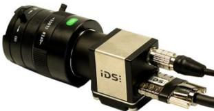
2. Please connect the Lemo connectors of the camera control cable with the Interface board of the W2100-System. The cable with the label „DIG IN“ connects to the „DIGITAL IN 1“ port and the cable with the label „DIG OUT“ to the „DIGITAL OUT 1“ port of the IFB-C Multiboot interface board.
