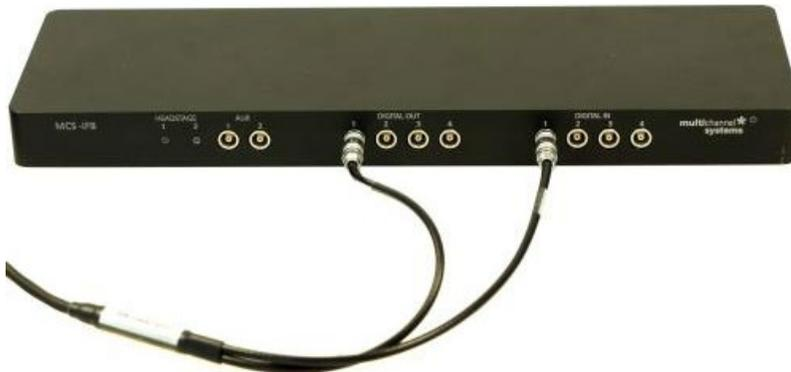
3. Finally connect the USB 3.0 to the computer. It is recommended to use an USB 3.0 port on the back side of the computer.
