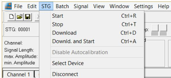
During the first ten minutes after starting the STG, the device emits every minute high frequency signals (small bursts) for internal offset calibration of the current outputs in a range of +/- 10 mV. After warming up the STG, the calibration signals later will be delivered half-hourly.
