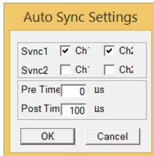
Assign the analog stimulus channels that will be used as the basis for autocreating the protocols on the Sync Out channels 1 and 2. For example, if you use only stimulus channel 1, select Ch1 under Sync1. If you use a MEA2100 amplifier, you can use up to two output channels per amplifier, that is, you may want to select Ch1 and Ch2 for Sync1.
