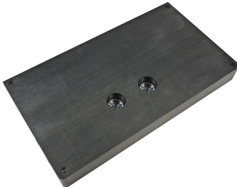
LED Stimulator for MEA2100-Systems with two slots for microelectrode arrays.
