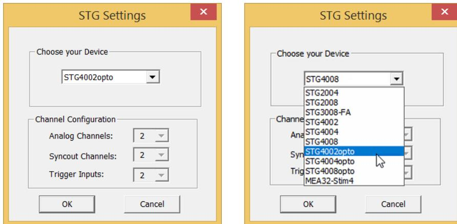
Please select the appropriate device type according to the connected STG from the drop down menu.
