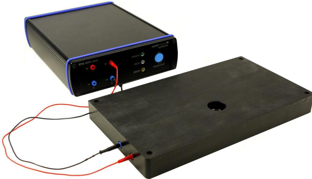
STG4002-1.6A-opto connected to a LED Stimulator for MEA2100-Systems with one slot for MEAs.
